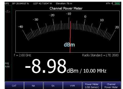
Power measurements over a defined bandwidth without an external sensor
